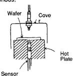
Fiber Optic Photoelectric Switch E3XR-CE4 (Amp) E32-T61 (Heat Resistant Fiber Unit - 300°C, Transmission Type)
