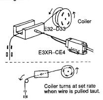
Fiber Optic Photoelectric Switch E3XR-CE4 (Amp) E32-D33 (Fiber Unit)
